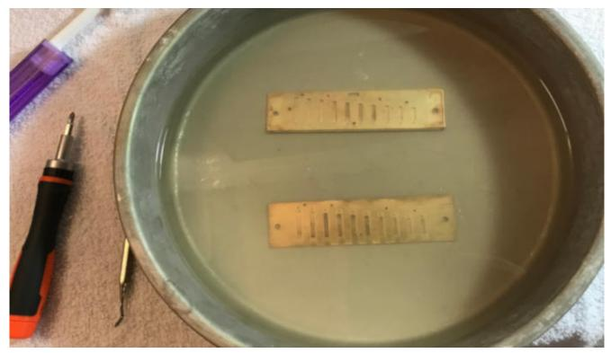
Soaking the reed plates in a lightly acidic solution for 15-30 mwithinutes helps loosen and split up any grime left on them from prolonged use. You need a light acidic solution that will do most of the cleaning, sufficient to interact with any kind of stray particles.
