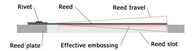
Embossing a reed slot is a narrowing of the slot in order to reduce the air loss around the sides of the reed. This can make the harp more air tight and increase the responsiveness of the reed. It can also help overblows to respond better.
