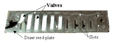
On harmonicas, "valves" are flaps attached to the reed plate at the rivet over the slot opposite the reed. See the picture above. They are made out of a thin plastic strip, or pair of strips, though they used to be made of other materials such as leather.
